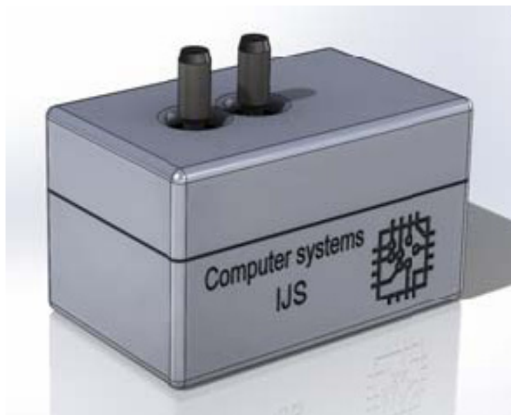
Figure 6. 3D model of the housing, which was printed using 3D printer and PLA plastic material
