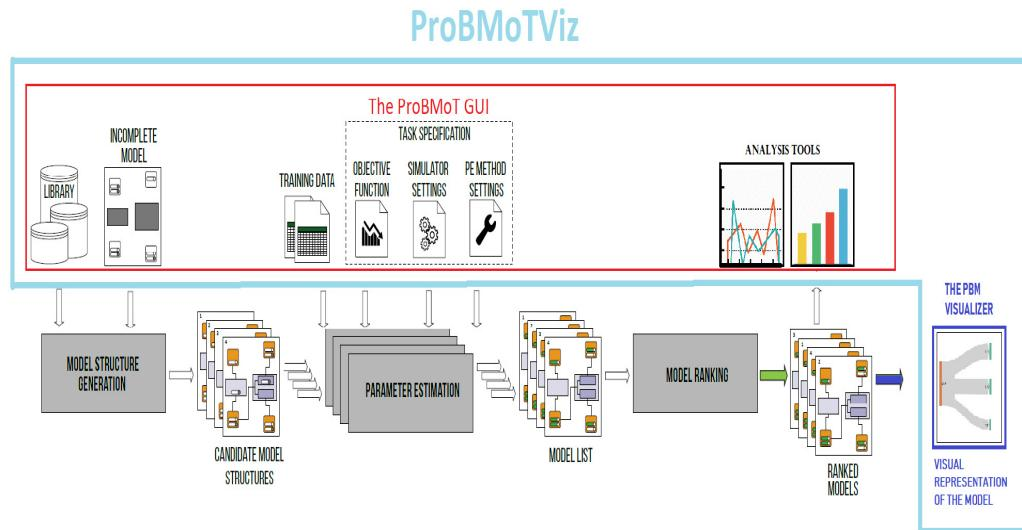
Figure 1. ProBMoTViz, the proposed extension of ProBMoT, consists of a GUI for ProBMoT and a PBM Visualizer
