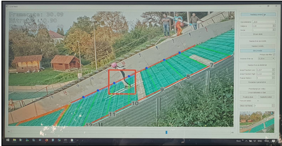
Figure 6. Trained operator determines the distance by using the calibrated measuring grid in 5-8
