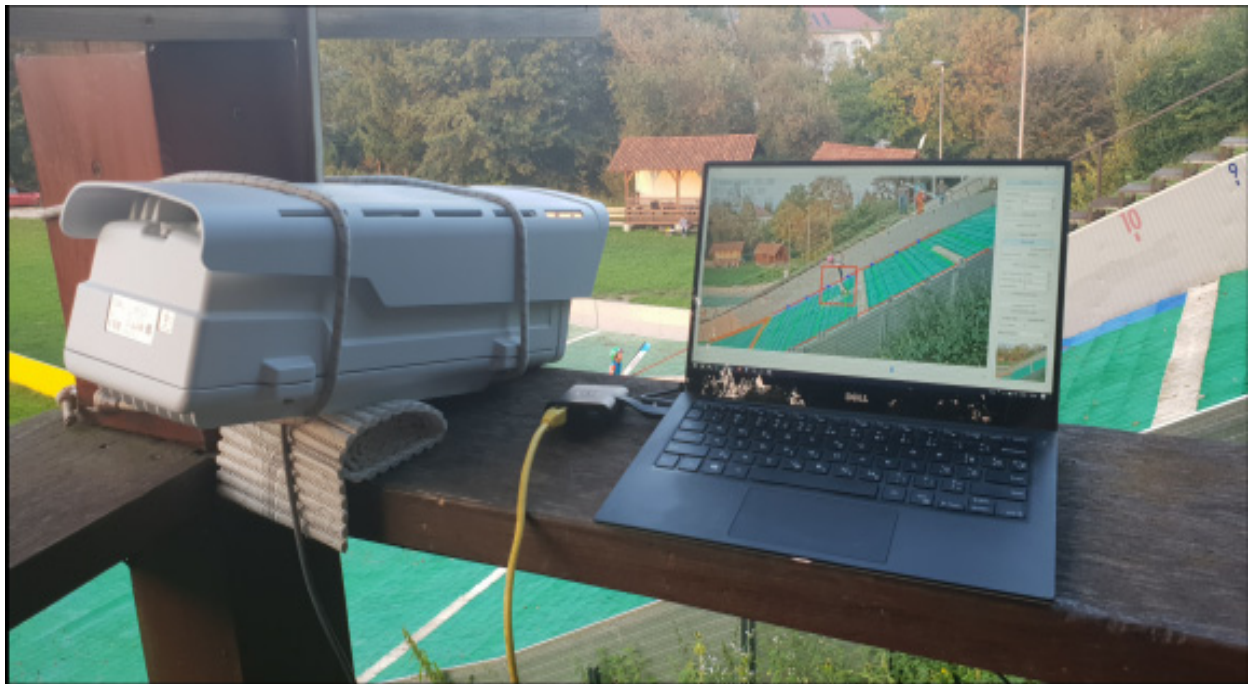
Figure 5. An online video distance measuring system consisting of a network camera (left) and a laptop computer
