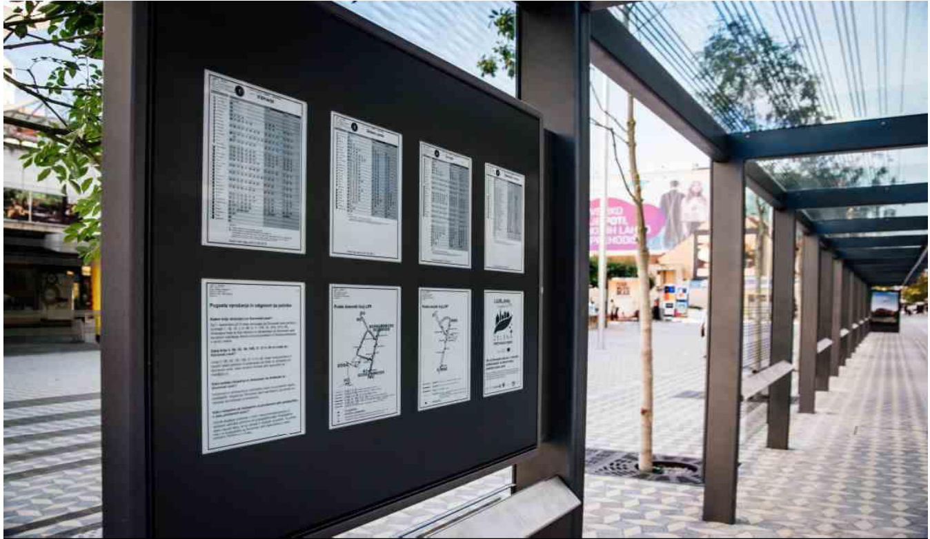
Figure 1. Digitizing existing city services: electronic paper displays with passenger information at Ljubljana’s bus stops
