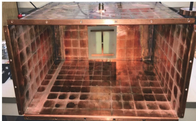
Figure 3. The dog-bone dipole structure in physical metal enclosure
