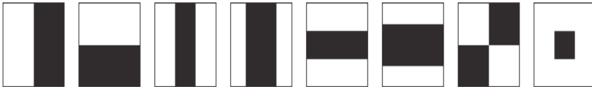
Figure 4. Eight type of masks are used for Haar-like feature extraction
