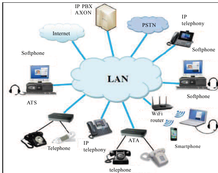
Figure 4. Axon IP PBX with integrated analog telephones by ATA Grandstream HT702
