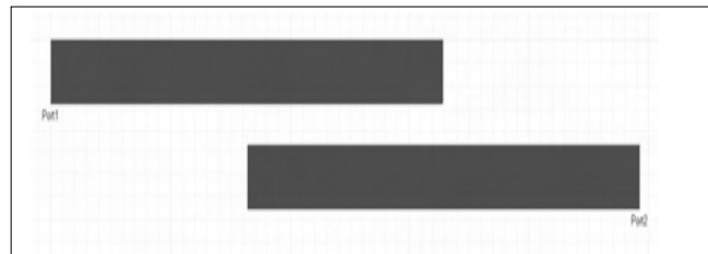
Figure 3. Two coupled resonators with length 32.82mm and width 2.76mm
