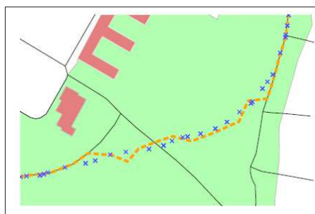
Figure 1. Example of a map with an embedded road network as well as free spaces and obstacles. The blue measurement-based trajectory is best explained by movement along the orange dashed path, which follows roads and free spaces where possible but contains no obstacle intersections
