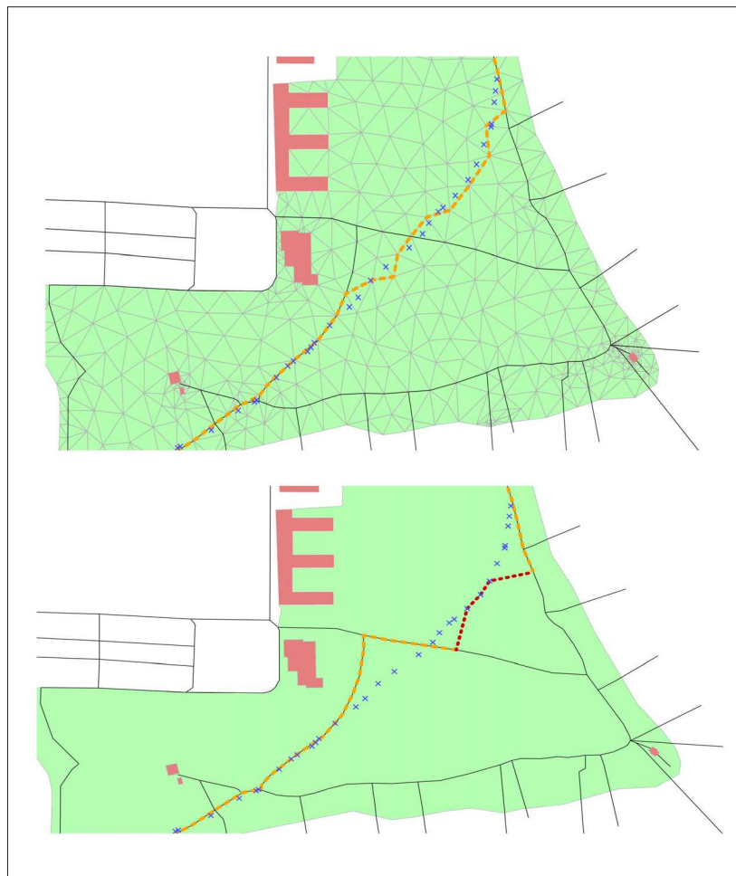
Figure 8. Original GPS measurements (blue crosses) and matched paths produced by the tessellation based approach (upper image) and Baseline+ (lower image). In the tessellation based matching the shape of the original trajectory is faithfully preserved and the unrestricted movement is correctly identified and matched to tessellation points and edges. Using Baseline+, the first part of the unrestricted movement is wrongfully matched to the path network and subsequently the shape is locally distorted when the switch from restricted to unrestricted movement occurs
