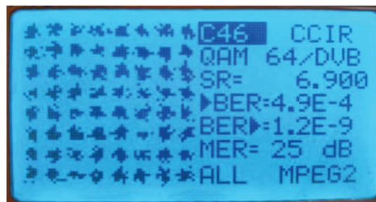
Figure 10. Constellation diagram for ch.46 with absence of disturbance
