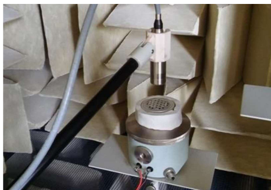
Figure 2. Measurement of transfer function of speech membrane in a small anechoic chamber using the coupler 2
