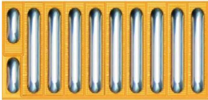
Figure 1. eGaN EPC2015C passivated die (size 4.6 x 1.6 mm)
