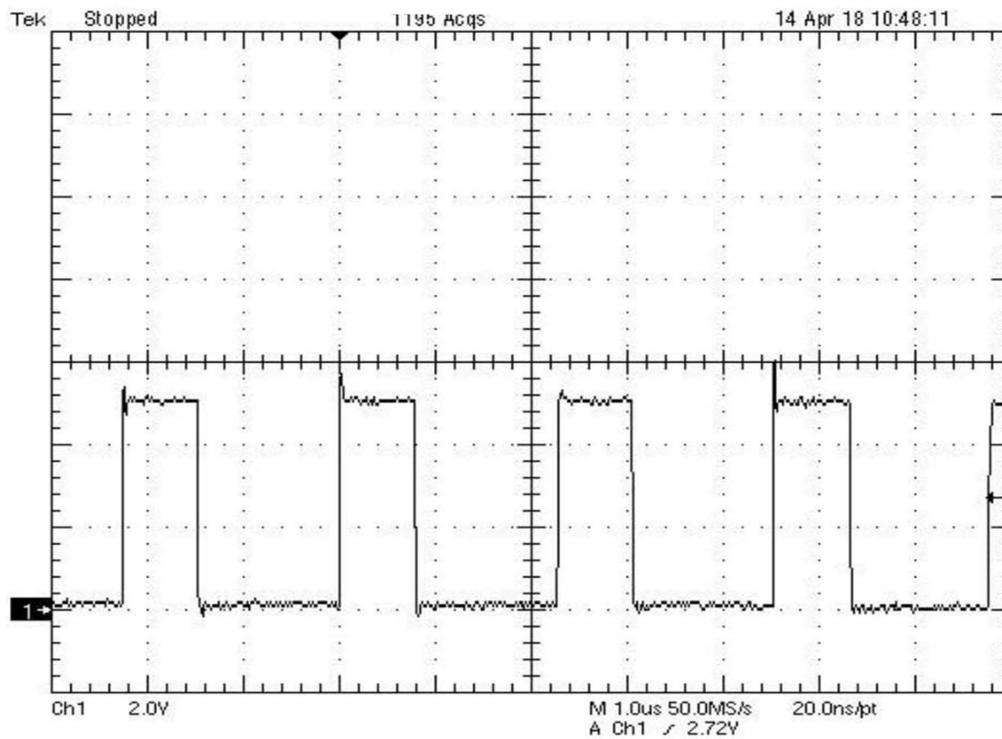
Figure 8. Gate voltage of low-side GaN FET
