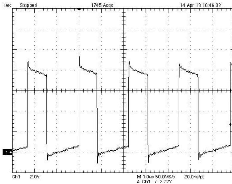
Figure 4. Drain voltage of high-side GaN FET
