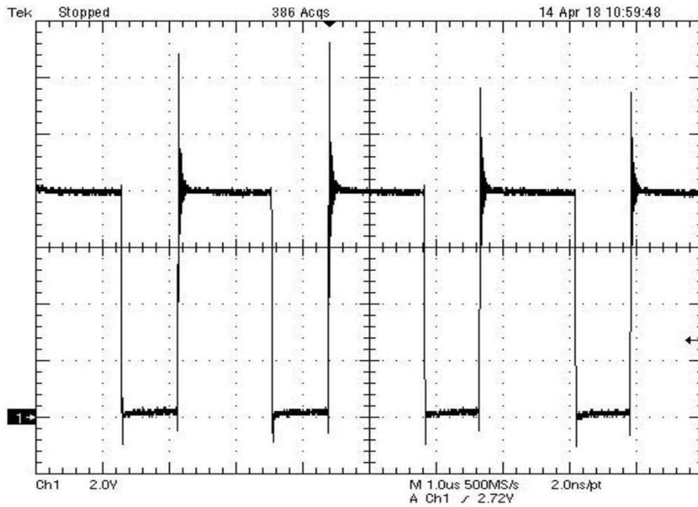
Figure 7. Drain voltage of low-side GaN FET
