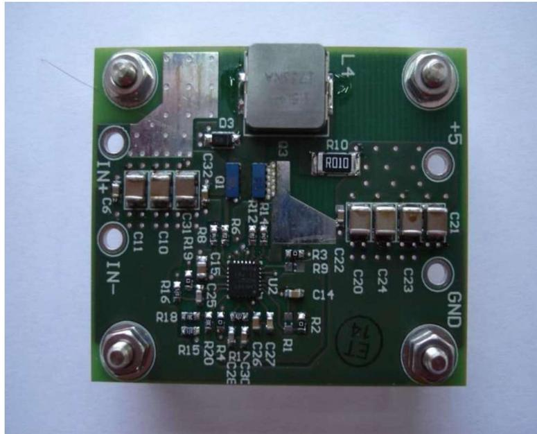
Figure 11. The converter prototype
