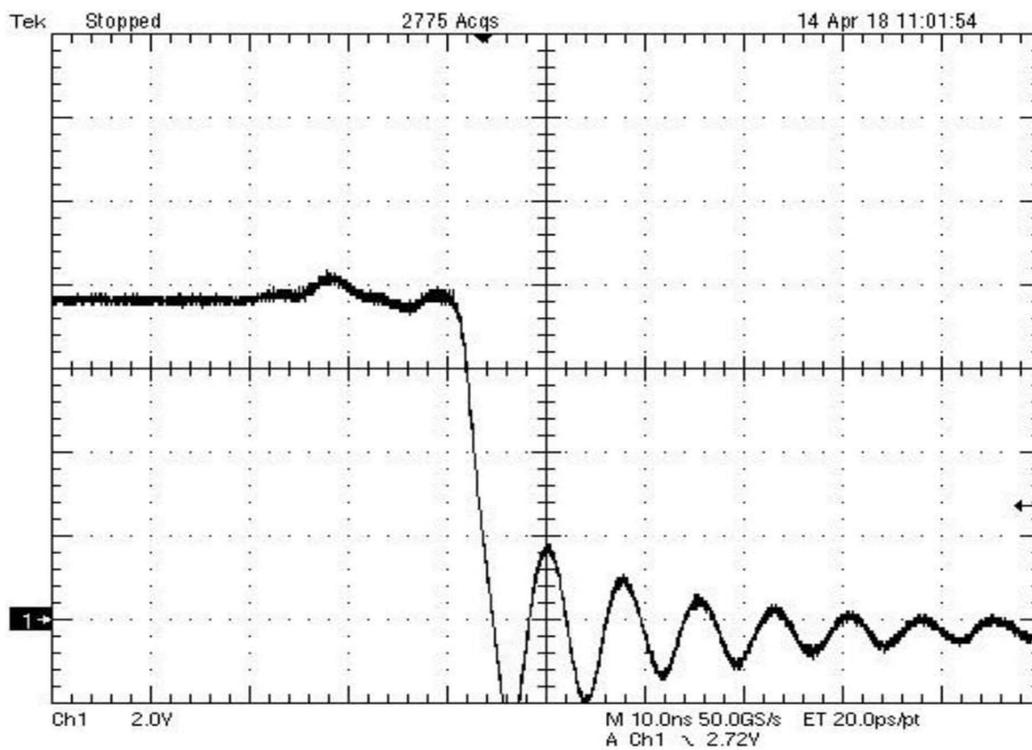
Figure 6. Turn-on waveform of high-side GaN FET
