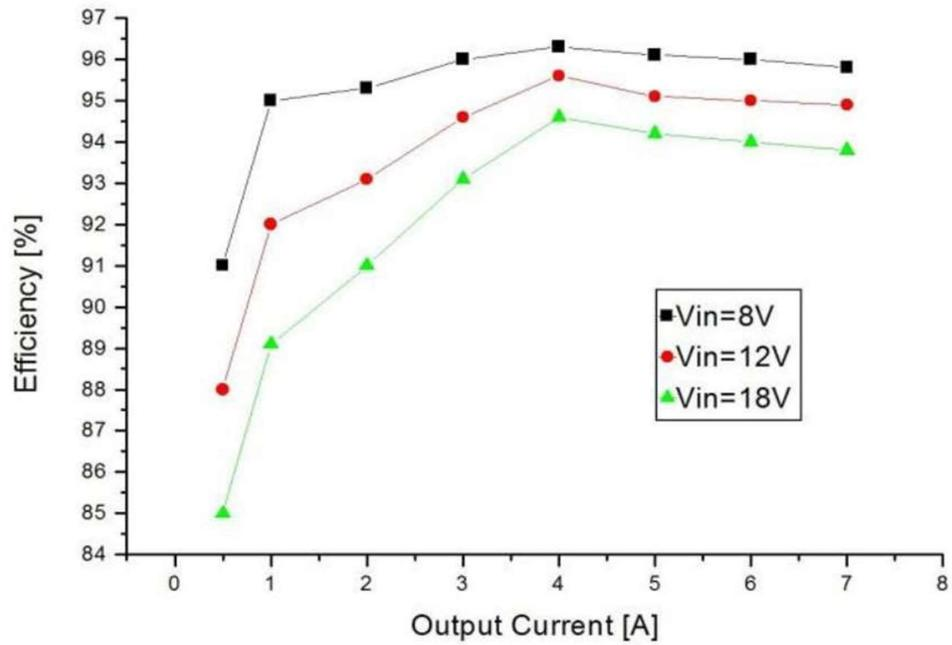
Figure 10. Measured efficiency vs. output current
