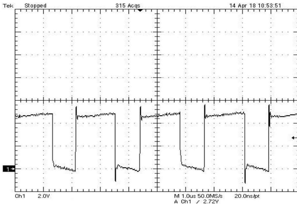
Figure 5. Gate voltage of high-side GaN FET
