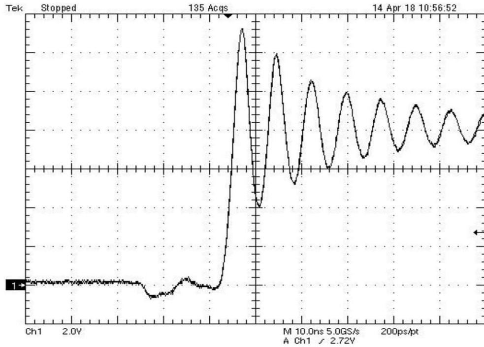
Figure 9. The ringing on the drain of low-side GaN FET at turn-off
