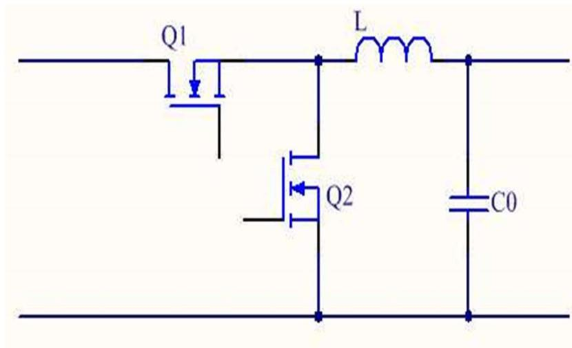
Figure 2. Synchronous buck converter
