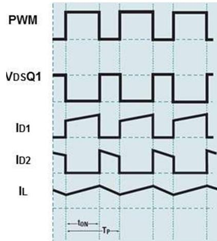
Figure 3. Synchronous buck converter waveforms
