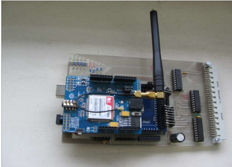
Figure 5. Arduino Mega interface board with the GSM module attached (Arduino SIM800C Module)
