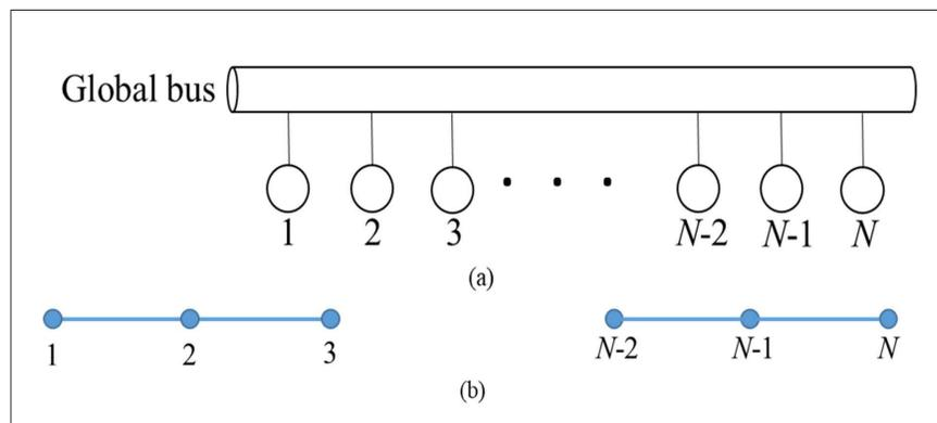
Figure 1. The bus topology modeled by a linear array graph
