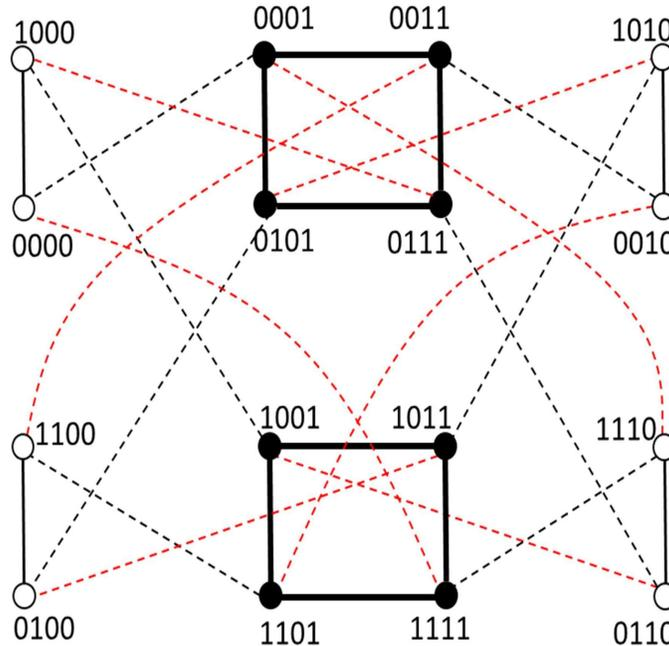
Figure 2. An exchanged folded hypercube  $EFH(1, 2)$
