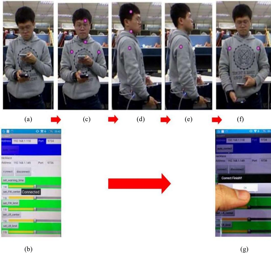
Figure 4. Using the notebook computer's image recognition function to calibrate the necklace's internal parameters
