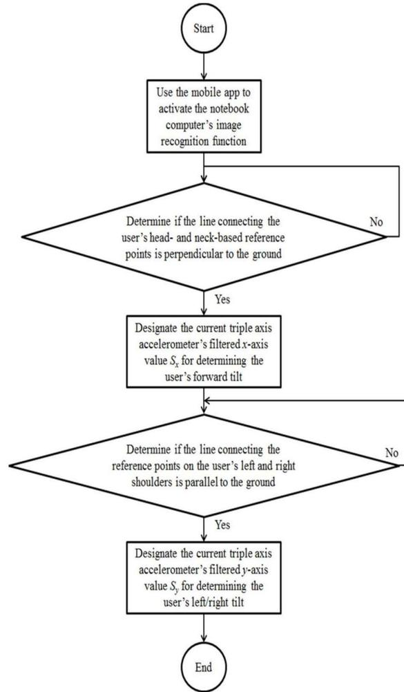
Figure 2. Flowchart of utilizing the notebook computer's image recognition function to calibrate the necklace's internal parameters
