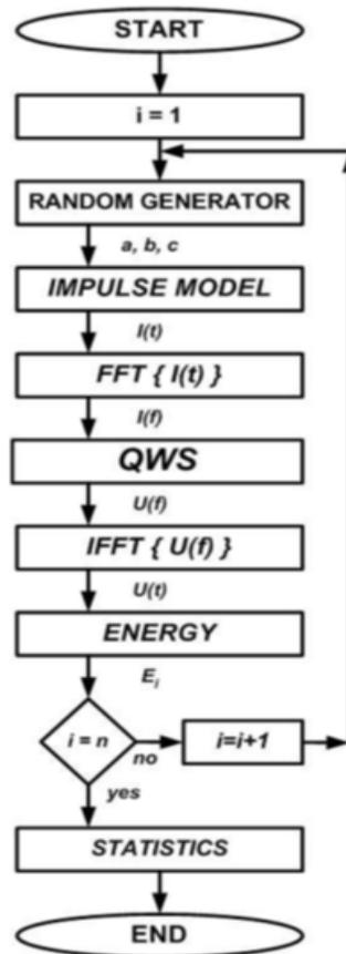
Figure 1. Block Diagram of the Algorithm
