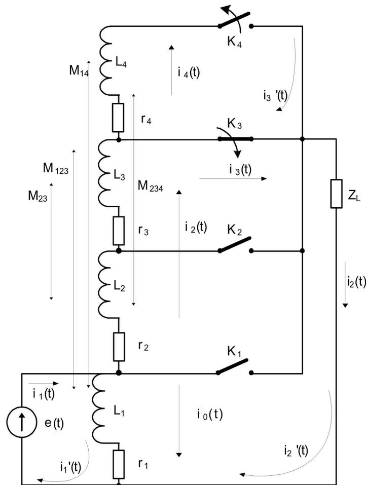
Figure 1. Equivalent Circuit of an ADACVR with Four CSS at Input Voltage Change
