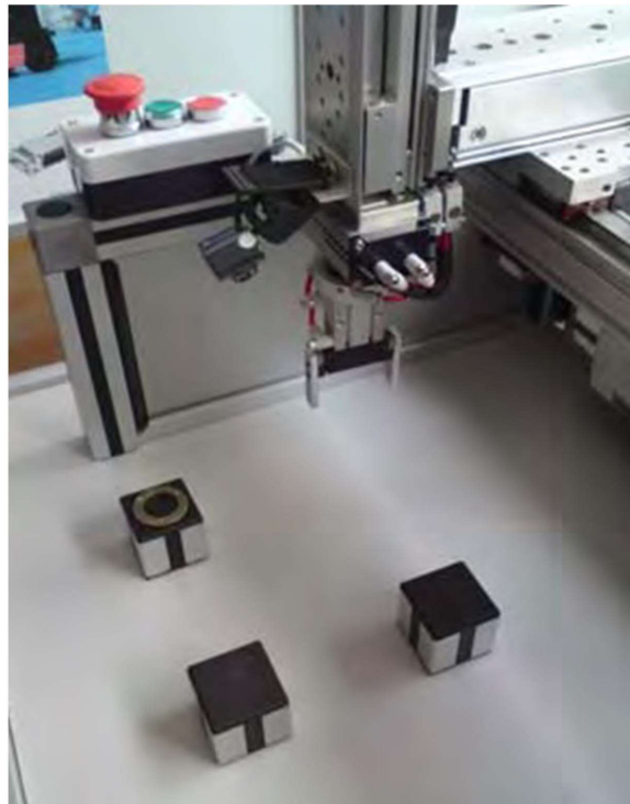
Figure 2. Experimental platform: 4-DOF manipulator with a moving camera
