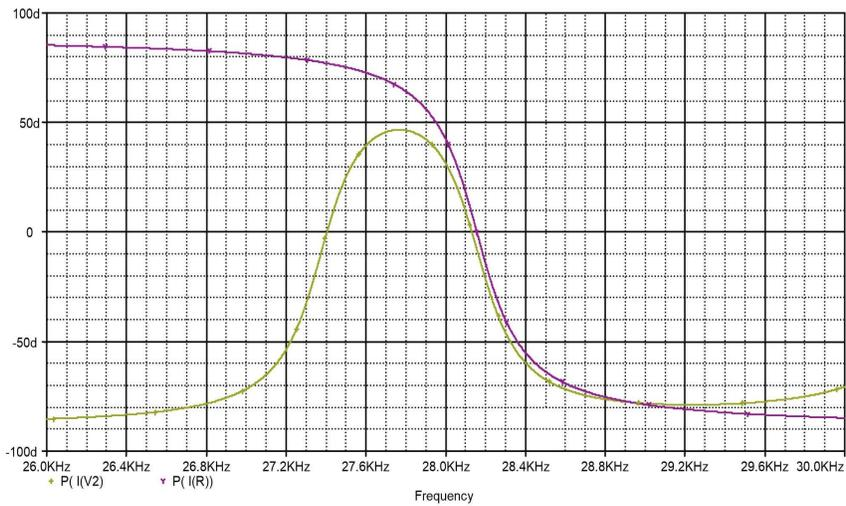
Figure 7. Phase-frequency characteristics of the generator  $P(I(V2))$  and CT currents  $P(I(R))$
