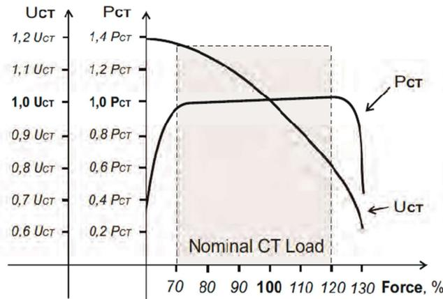
Figure 9. Load characteristics with the control system being switched on
