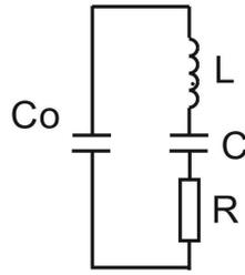
Figure 4. Basic scheme of piezoelectric CT
