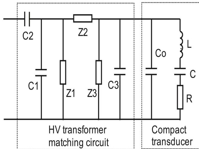
Figure 5. HV transformer, matching capacitors and CT equivalent circuit
