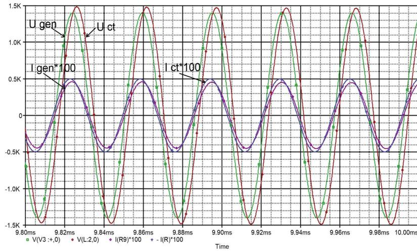
Figure 6. Waveforms of the voltages  $U_{gen}$ ,  $U_{ct}$  and currents  $I_{gen}$ ,  $I_{ct}$
