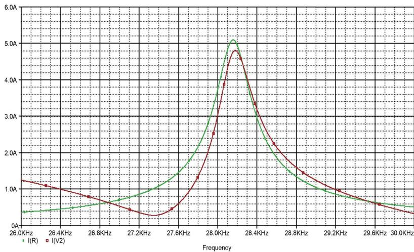
Figure 8. Amplitude-frequency characteristics of the generator  $I(V2)$  and CT currents  $I(R)$
