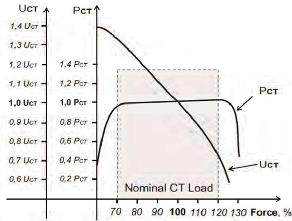
Figure 10. Load characteristics with the control system being switched off
