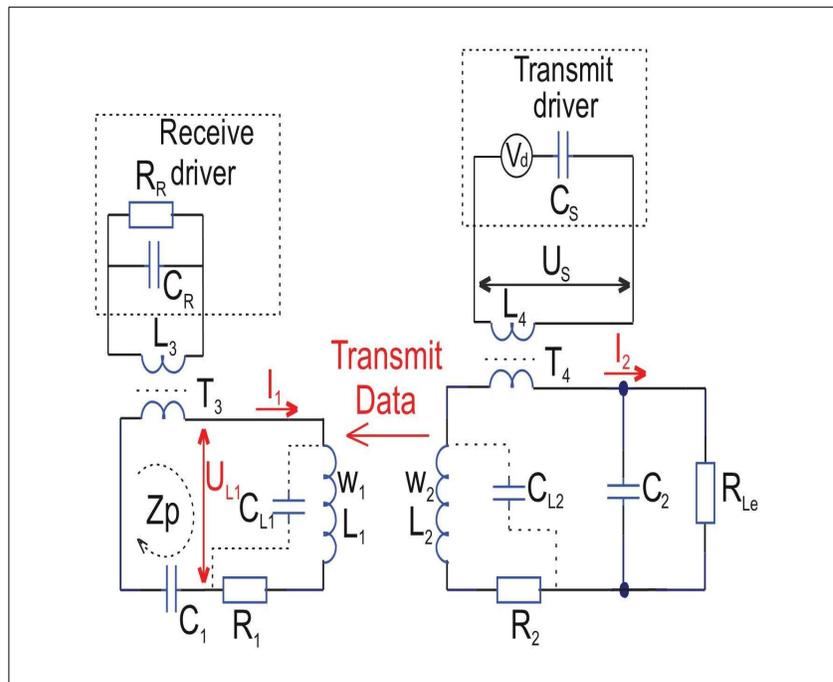
Figure 3. An equivalent scheme used to transfer data from the power transmitter to the receiver
