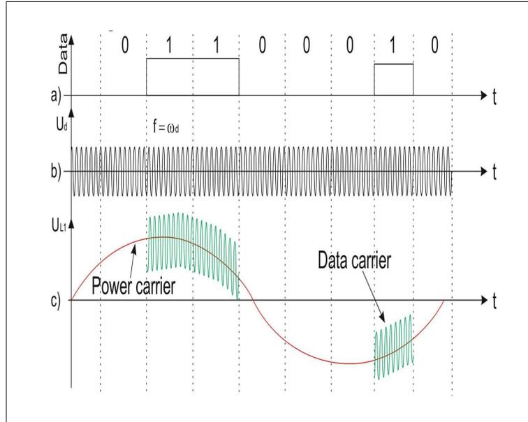
Figure 2. a) The chart of the transmitted information signal; b) The used data carrier frequency  $\omega_d$ ; c) The received signal from the overlaid frequency for transmitting energy and the frequency of data transmission
