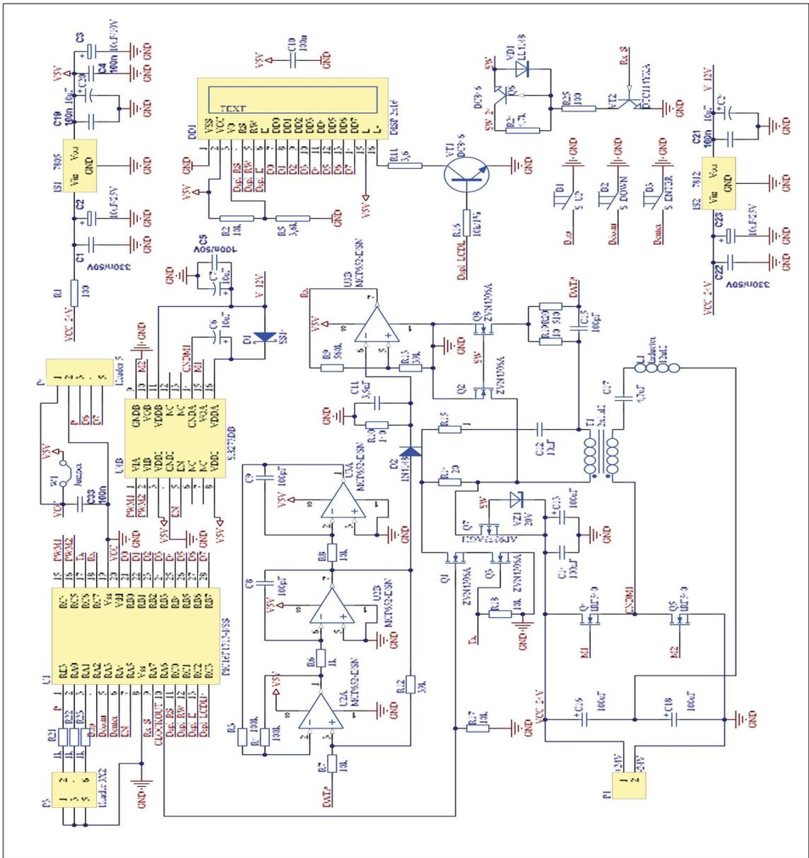
Figure 7. Scheme of the wireless power transfer and the data transmitter and receiver
