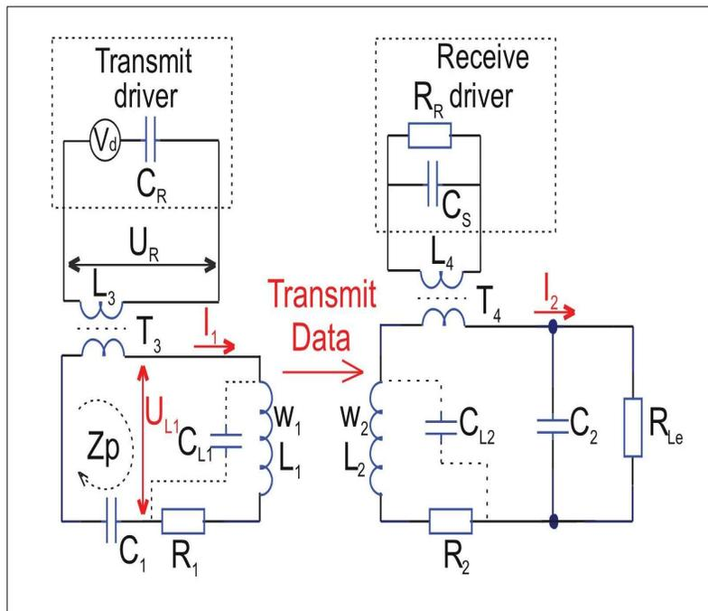
Figure 1. An equivalent scheme, used to transfer data from the power transmitter to the receiver
