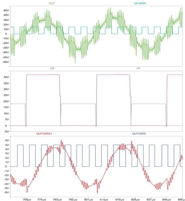
Figure 6. Computer simulation results at data transfer from the receiver to the transmitter: U2-DATA-voltage of transmitted energy from the receiver, OUT – voltage of transmitting data winding; U5 and U6 - transistor M1, M2 gate voltage control; OUTDATA1 - strip filter; OUTDATA - voltage of received data.
