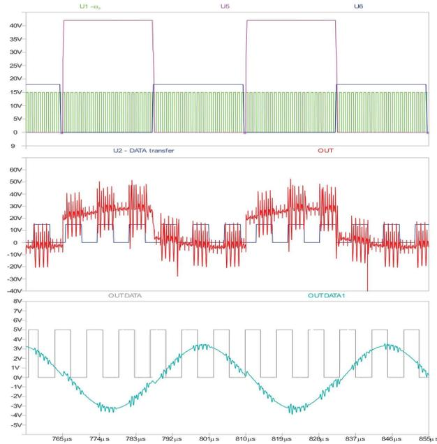
Figure 5. Computer simulation results at data transfer from the transmitter to the power receiver: U1 – data transmission voltage with frequency of  $\omega_p$ ; U5 and U6 - the transistor M1, M2 gate voltage control; U2 - the voltage of the transmitted data; OUT - the voltage at the resonant inverter circuit; OUTDATA1 - the voltage at the receiving data coil; OUTDATA - the voltage of the data formed in the receiving part.
