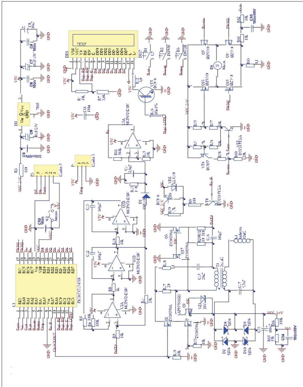
Figure 8. Scheme of the energy receiver, and the data transmitter and receiver
