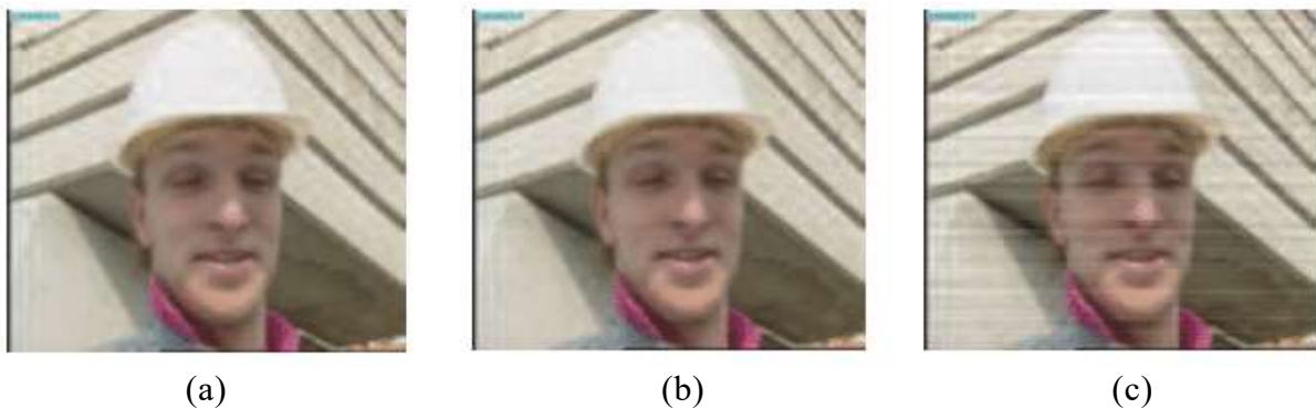
Figure 5. The first frame of the video coded by H.264 codec where the watermark with a) \alpha=0.005 b) \alpha=0.01 c) \alpha=0.05 was inserted
