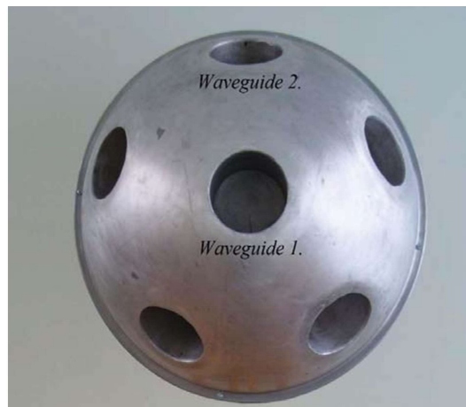
Figure 7. Photo of the developed laboratory model of aperture antenna array: W1 - \alpha_1=0 deg and \beta_1 = 0 deg; W2 - \alpha_2= 56 deg and \beta_2 = 180 deg; r_w = 6 cm; r_s = 30 cm
