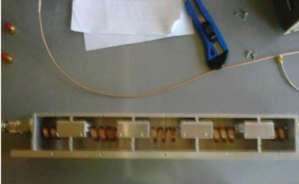
Figure 8. The produced VHF low pass filter
