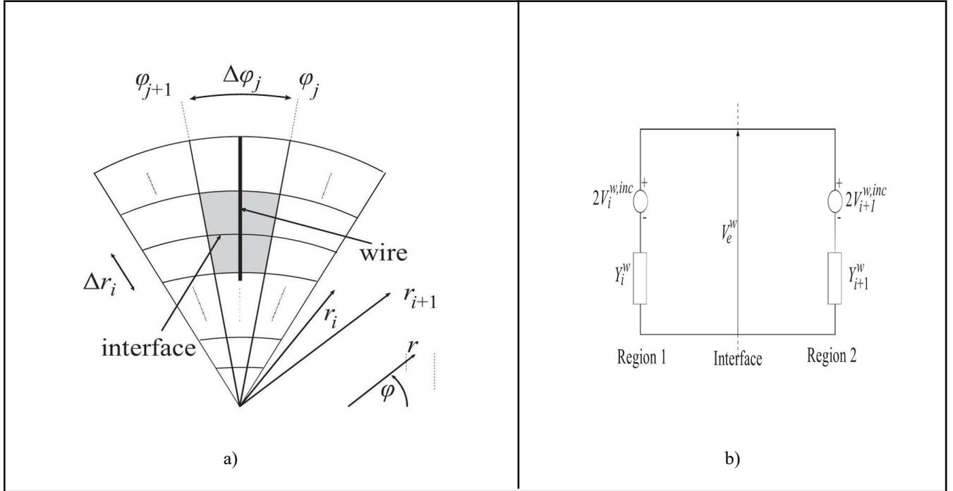
Figure 2. a) TLM nodes in  $r\phi$  plane through which wire runs and b) an interface between two nodes
