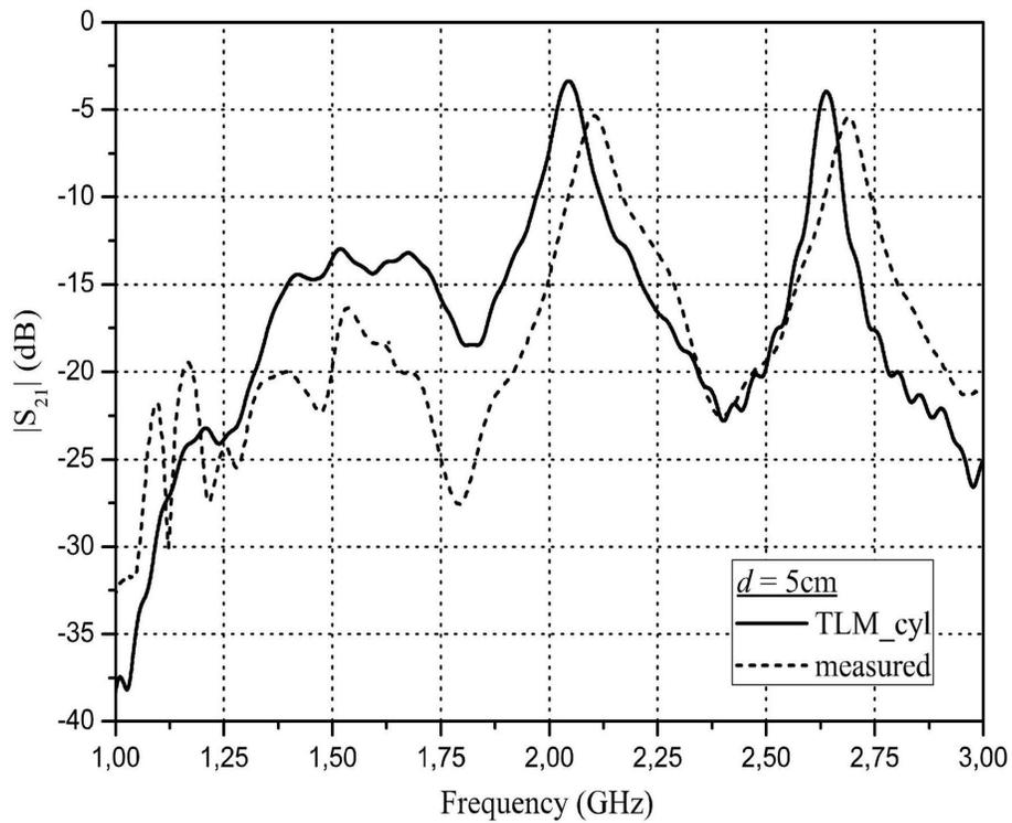
Figure 4. Transmission coefficient magnitude in the cylindrical cavity loaded with one water layer
