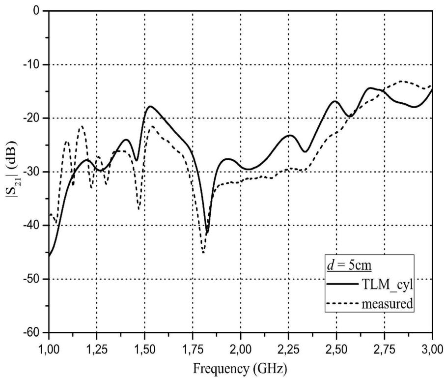
Figure 5. Transmission coefficient magnitude in the cylindrical cavity loaded with two water layers
