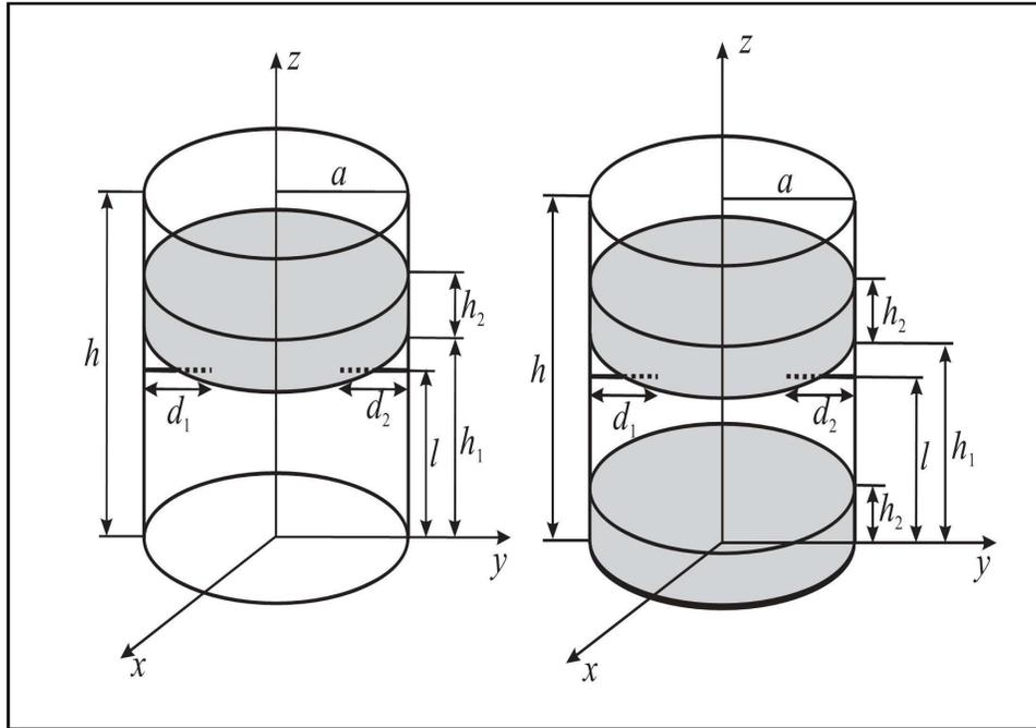
Figure 3. A probe-coupled loaded cylindrical cavity with a) one water layer and b) two water layers
