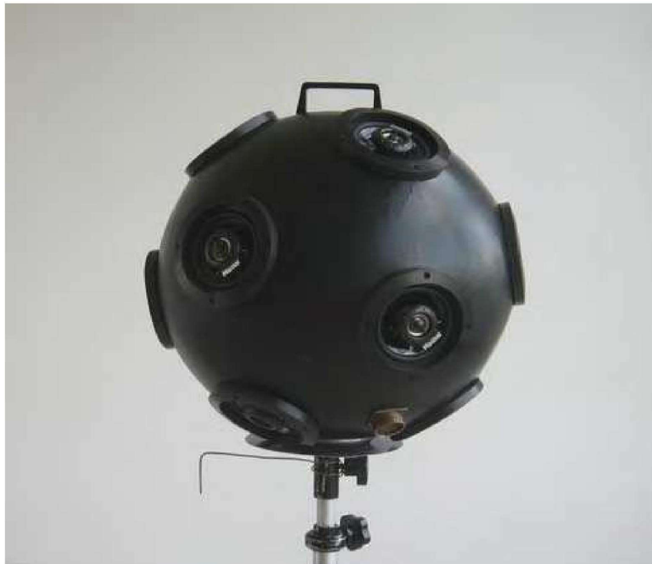
Figure 1. Sound source with independent elements (loudspeakers) in the form of a dodecahedron
