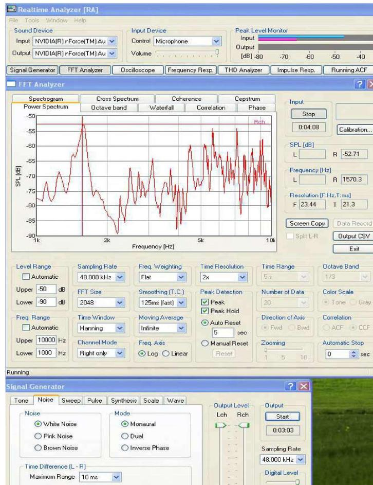
Figure 4. The measured sound pressure in the closed cylindrical enclosure (dimensions: height 6.2cm, diameter 13cm and wall thickness 0.1cm)
