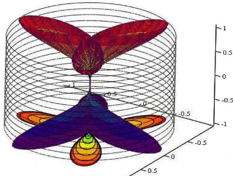
Figure 2. Distribution of the magnitude of sound pressure in a cylindrical box:  $j$  axial sound wave,  $f = 3.538$  kHz,  $j = 3$ ,  $k = 0$ ,  $\lambda_{j,k} = 4.201189$ ,  $\cos(j \cdot \theta)$ , mode (0, 3, 0)
