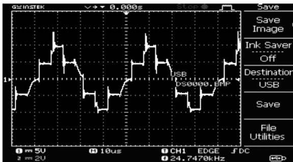
Figure 38. Experimental five level inverter output voltage
