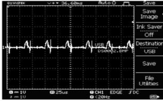
Figure 42. Experimental isolation transformer output voltage
