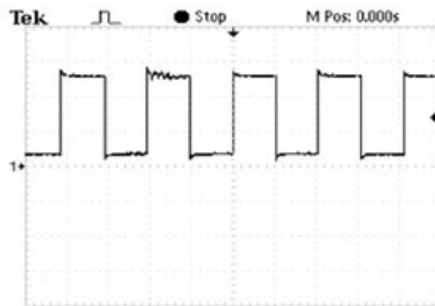
Figure 53. Gate signal for switch S1
