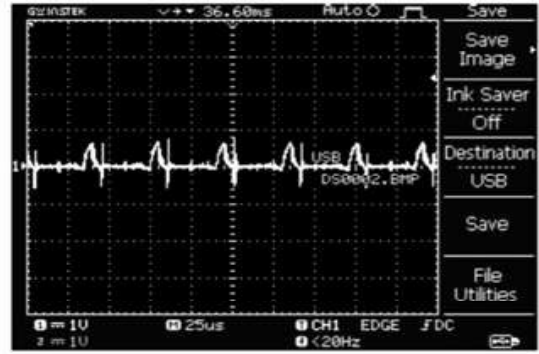
Figure 43. Experimental isolation transformer output current
