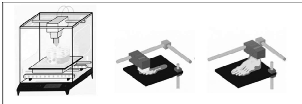
Figure 1. 3D printing technology forming principle diagram
