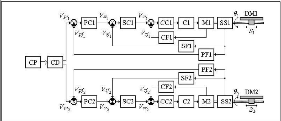
**Figure 1. Block diagram of the two-coordinate drive system**
