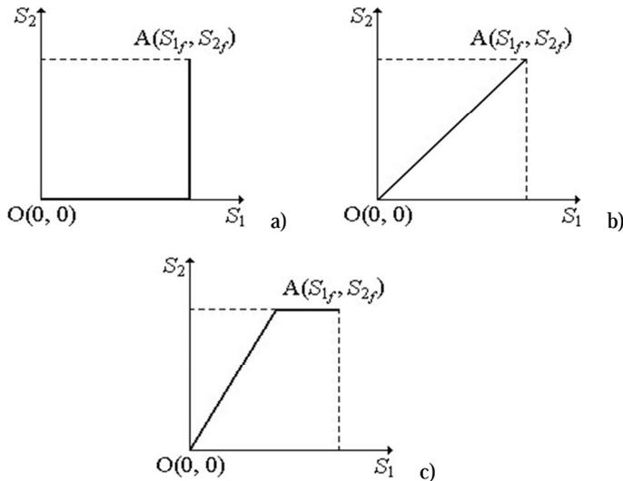
Figure 2. Motion trajectories for two-coordinate position control
