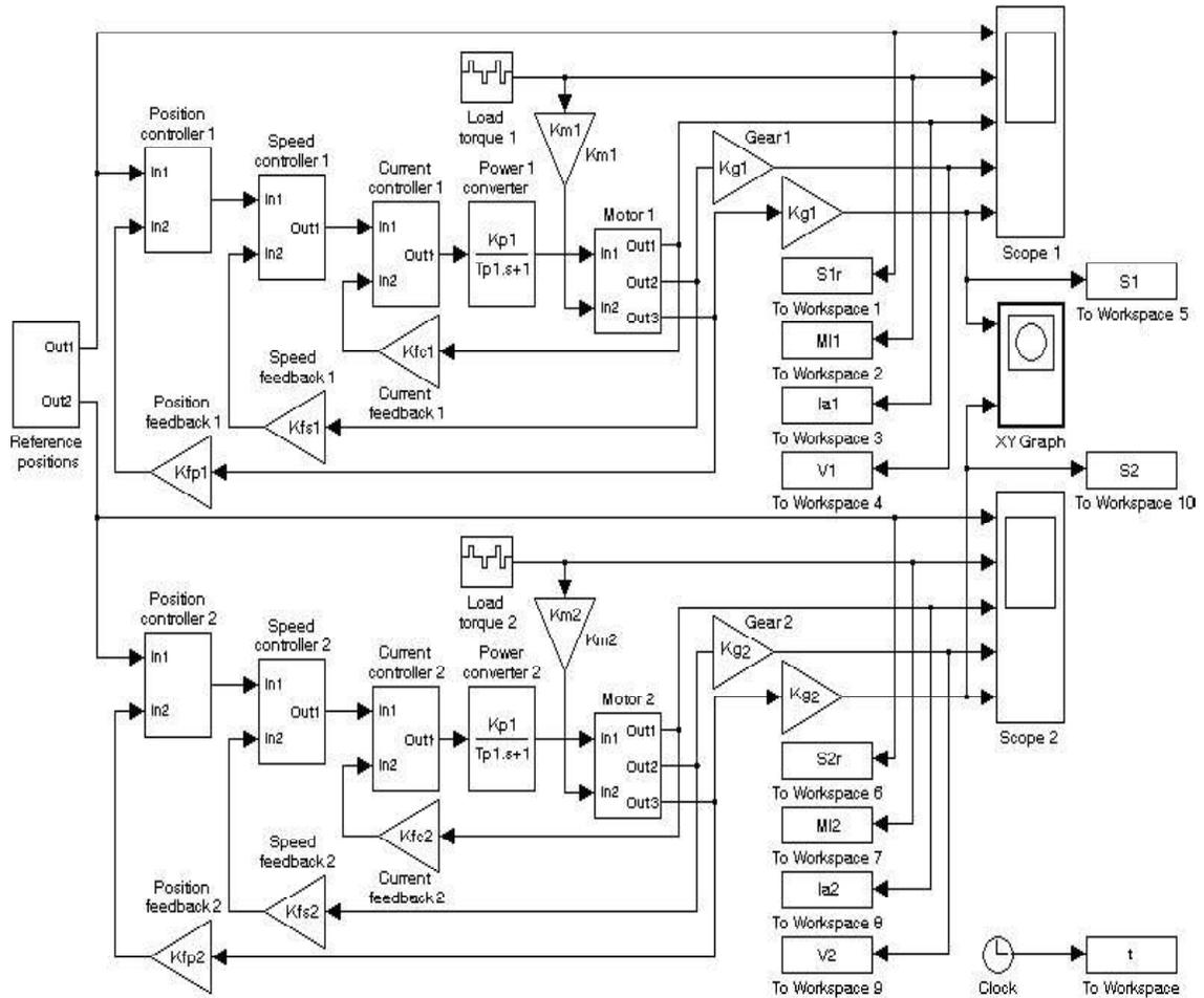
**Figure 3. Simulation model of the two-coordinate drive system**
