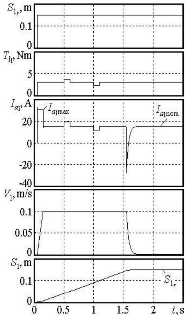
**Figure 4. Time-diagrams for a set position cycle along one axis**
