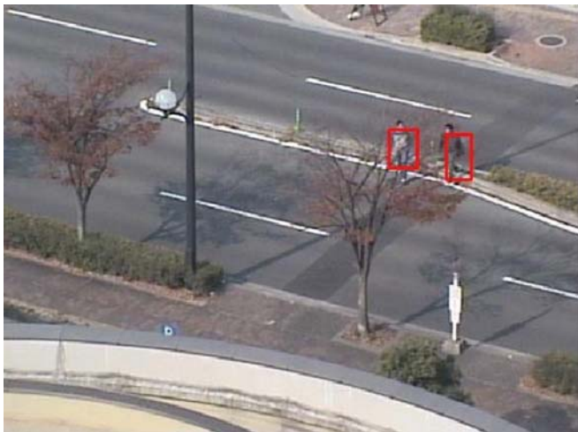
Figure 3. Detection of Intrusion at the Specific Place: it is judged that there is no intruder
