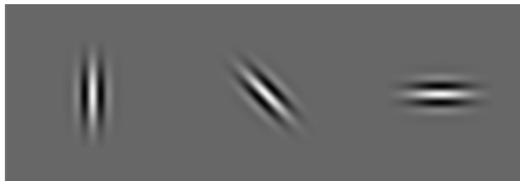
Figure 5. A bank of Gabor filter oriented respectively 0^\circ , 45^\circ and 90^\circ
