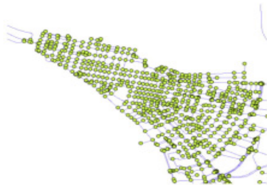
Figure 3. A graph associated to a selected area of the city, each node is a road intersection and each branch is the segment that connects two intersections
